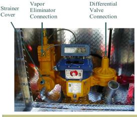
LC electronic meter shown. Mechanical registers will not have the 3rd line from the register head to the vapor eliminator.
